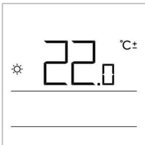
Press the  $+$  or  $-$  button to activate the setup of the desired daytime temperature. Buttons  $+$  and  $-$  change the desired temperature. Press the  $i$  button to return to the home screen.
