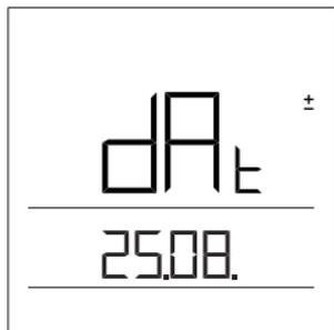
Press the  $+$  or  $-$  button to activate the setup of the desired daytime temperature. By pressing the  $i$  button three times you move to the date display. By pressing the  $+$  or  $-$  button and holding it for at least 2 seconds, the time value starts flashing and you can change it with the buttons  $+$  and  $-$ . Move to other settings by pressing the button  $i$ . Set the hour, minutes, day, month, and year. Press the  $i$  button to return to the home screen.
