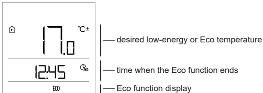
Now you can change the desired low-energy temperature with the buttons **+** and **-**. The value is flashing during the setup process. Press the **Eco** or **i** button to move to time setting. The buttons **+** and **-** are used to configure how long the Eco function shall remain active. The value is flashing during the setup process. Press the **ECO** or **i** button again to return to the home screen.
