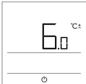
Press the  $+$  or  $-$  button to activate the setup of the desired daytime temperature. Press the  $i$  button twice to move to the frost protection temperature display. By pressing the  $+$  or  $-$  button and holding it for at least 2 seconds, the setting value starts flashing and you can change it with the buttons  $+$  and  $-$ . Press the  $i$  button to return to the home screen.
