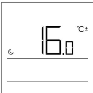
Press the  $+$  or  $-$  button to activate the setup of the desired nighttime temperature. Press the  $i$  button to return to the display of the desired nighttime temperature. Buttons  $+$  and  $-$  change the desired temperature. Press the  $i$  button to return to the home screen.
