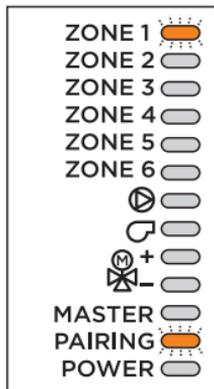
The pairing process determines which zone will be affected by the room unit being paired. A room unit that has not been paired yet only displays the measured room temperature. The pairing process must first be activated on the controller where the LED lights indicate which zone is currently being paired.
