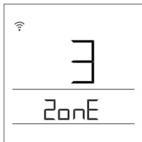
After the pairing process is successfully completed, a beep can be heard and the number of the zone to which the room unit has been connected is displayed for 5 seconds. The controller automatically switches to pairing the next (unpaired) zone.
