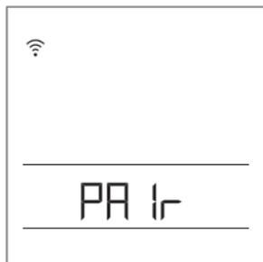
If the room unit should affect the signalled zone, the pairing process is activated on the room unit as well by holding the buttons + and - for 2 seconds. During the pairing process, "PAIR" is displayed.
