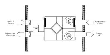
During normal operation intake and discharge dampers will be open while the recirculation damper will be closed.
