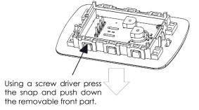
Connections shall be in compliance with existing rules and using max 2,5mm<sup>2</sup> cross section wires for J1 and J2 terminals and 1,5mm<sup>2</sup> cross section wires for J3 and J4.
