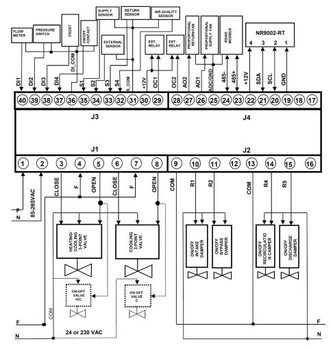
The controller operates through the parameters storaged inside which can be modified using the remote sensor NR9002-RT or through the supervisory system (MODBUS protocol). The remote sensor NR9002-RT allows to set and visualize the following parameters:
