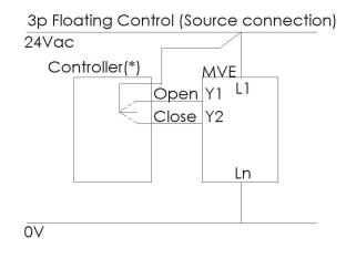
Matching between MVE terminal block and others Controlli actuators
