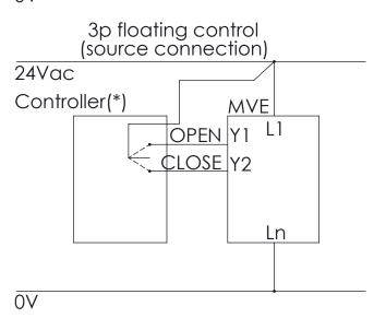
(\*) MVER contain a half-wave rectifier power supply. They must not be powered with transformers that are used to power other devices using not isolated full-wave rectifier power supply.
