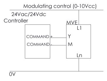
N.B.: M and Ln signal are internally connected
