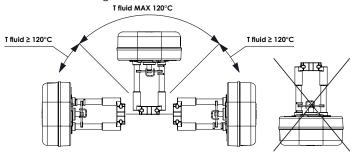
To mount the actuator on to a valve, position the valve stem to the bottom of its travel, slide the actuator onto the valve neck, adjusting with the manual override the screw jack position so the square nut on the valve spindle fits into the groove on the cross bar. Then slide the brace into the groove on the valve neck and secure the nuts.
