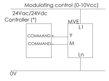
N.B.: M and Ln signals are internally connected.
