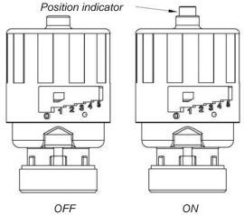
The actuators complete the stroke when the pin exceeds the cover collar by 4mm.
